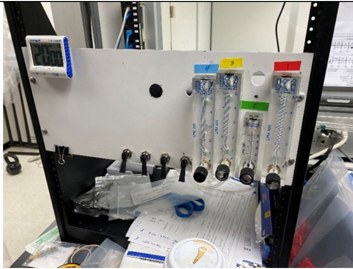
Figure 1-2. Sample collection manifold constructed with four Key Instrument Rotometers and a Gast DOA P707-AA vacuum pump.
