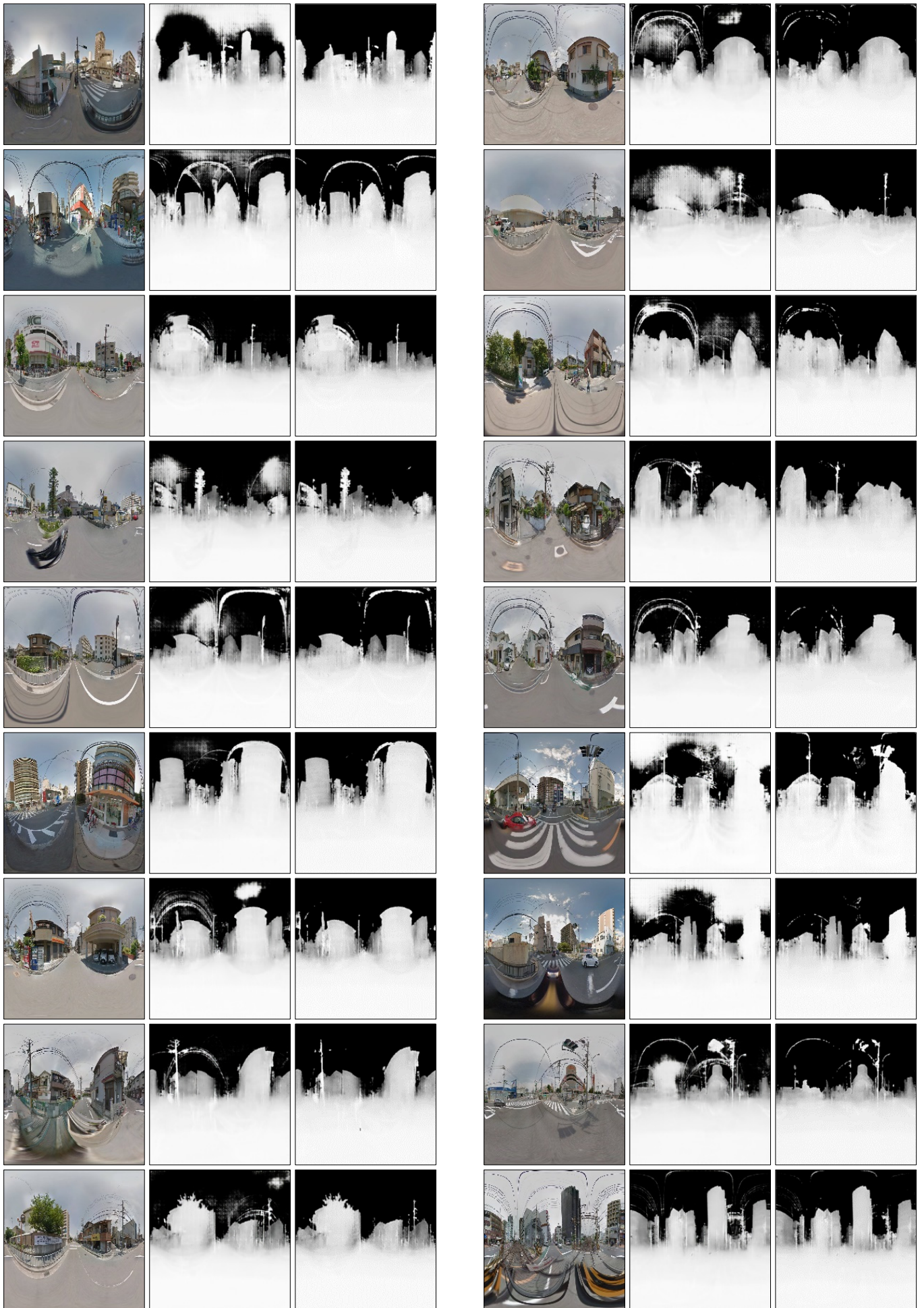
Figure 1. All 100 depth maps of GSV generated by M2c and their filtered images: Omnidirectional image (©Google, left), generated depth map (center) and filtered depth map (right), part 1/6
