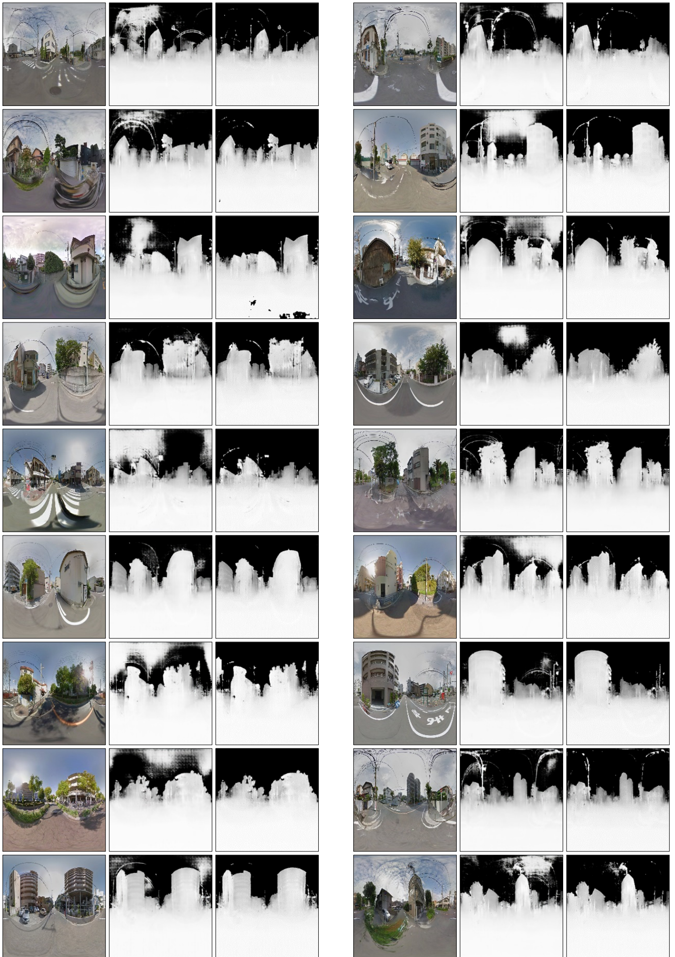
Figure 5. All 100 depth maps of GSV generated by M2c and their filtered images: Omnidirectional image (©Google, left), generated depth map (center) and filtered depth map (right), part 5/6
