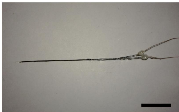
Fig. S11. Optical image of gel-electrolyte coated two-ply asymmetric supercapacitor. The overall diameter is about 350\ \mu\text{m} . (scale bar = 1\ \text{cm} )
