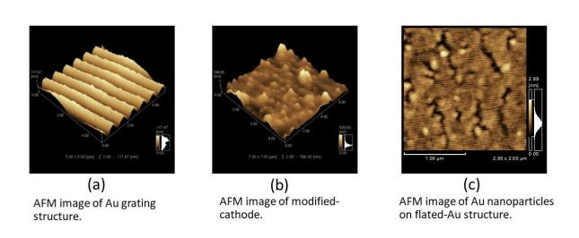
**Figure. S1.** Atomic-force microscopy images of (a) the gold-coated grating layer, (b) the overall structure of the modified cathode, and (c) AuNPs on a flat gold structure.
