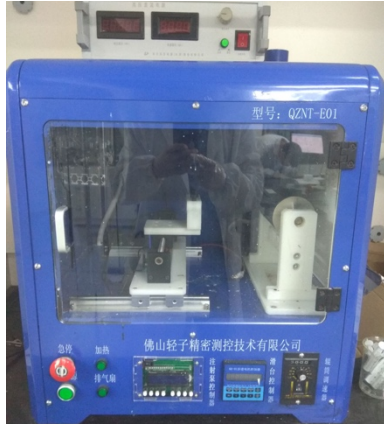
Figure SI-1. Photograph of QZNT-E01 electrospinning apparatus. Front view of apparatus cabinet (safety enclosure) and front control panel and digital high-voltage supply illustrated resting on top of cabinet. Through the front window are visible the cylindrical collector drive on right, the needle holder and back and forth rastering-assembly (middle), and syringe drive partially visible in upper left corner of window.
