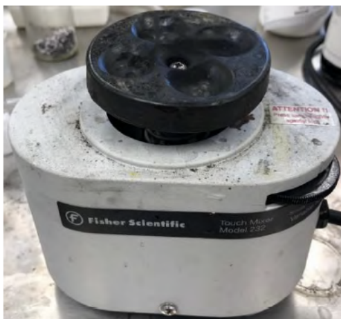
Figure SI-1. Fisher Scientific vibrator stirrer used for low-shear mixing applications in this study.
