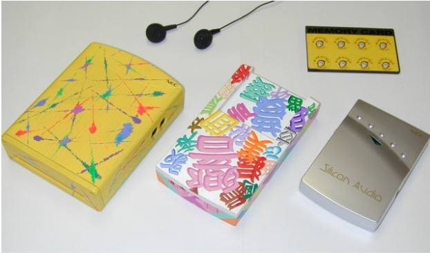
Fig. 6. Three generations of the Silicon Audio developed in early 1994 [13], late 1994 [14], and 1997 [15] (Left to right).
