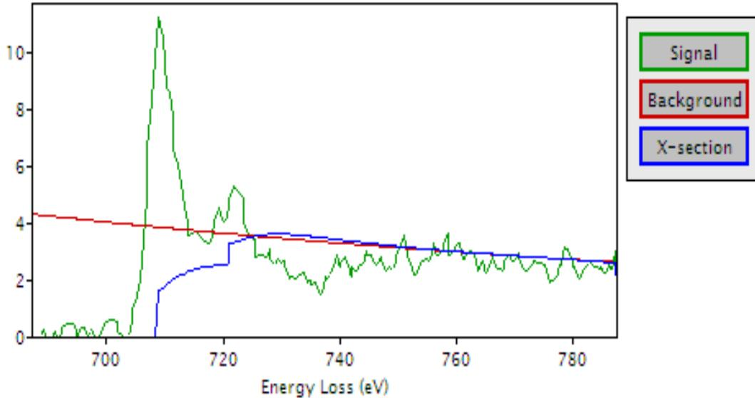
**Figure A.** Typical spectrum from particle and calculated H-S Cross-section
