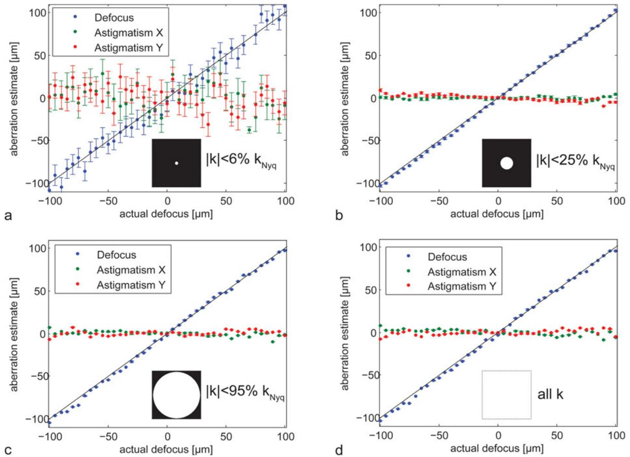
**Supplementary Figure 1.** Influence of the spatial frequency range used in MAPFoSt analysis. A given through-focus series of experimental images analyzed using (a) spatial frequencies  $|k| < 0.06 k_{Nyq}$ , (b)  $|k| < 0.25 k_{Nyq}$ , (c)  $|k| < 0.95 k_{Nyq}$ , (d) all spatial frequencies.
