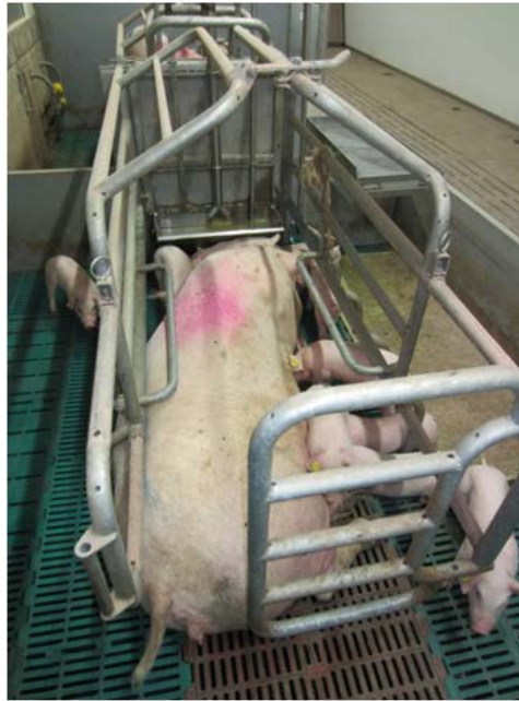
Figure 2: Knick pen (BRÄUER Stalltechnik, Behamberg, Austria): plan of pen with open crate and photograph of sow in closed crate. Both side elements of the crate adjustable in length (telescopic design), one in width. Flexibly pivoted door in the back for closing the crate. Lowest bars (distance to floor: 0.35 m) equipped with vertical pins of half-round, convex shape with tips directing towards the floor. Flooring: solid concrete floor (creep area in beige and area in front of the trough in light grey), cast iron slatted floor (red), plastic slatted floor (light green) and plastic partially slatted floor (dark green). Farrowing rails attached to the rear and one side wall of the pen.
