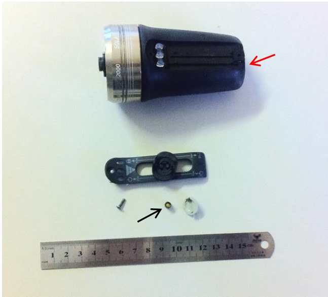
Fig. 2: The switch of the Sola 2000 light disassembled. The black arrow indicates the magnetic switch. The red arrow indicates the position of the overpressure valve.
