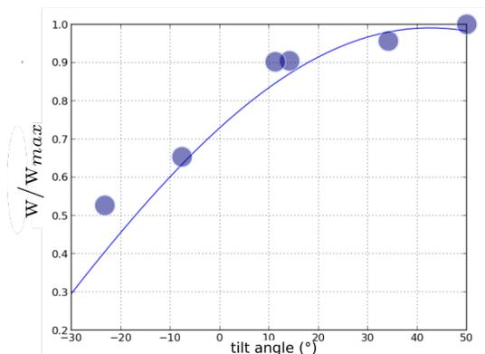
Figure 1: a) Analysis of the contrast of dislocations  $d_1$  and  $d_2$  in dark field mode . b) is the stereographic projection of the wire. c) is the theoretical variation of the apparent dislocation width with the tilt angle in the basal plane and experimental measurements (dots).
