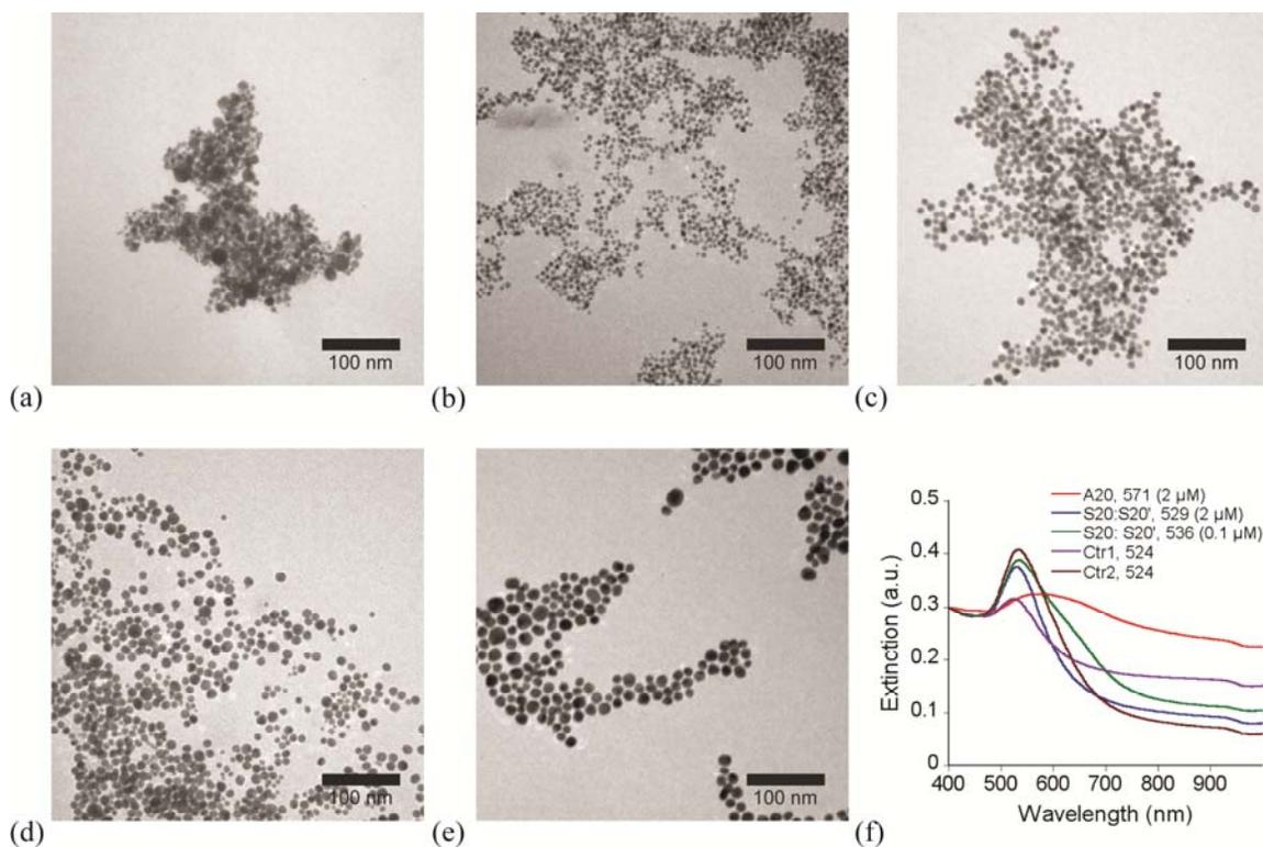
**FIG. S1.** TEM micrographs of gold seed aged for 7 days in the presence of added (a) A20 at 2  $\mu\text{M}$  (b) S20:S20' at 2  $\mu\text{M}$  (c) S20:S20' at 0.1  $\mu\text{M}$  (d) 2  $\mu\text{L}$  Tris HCl (Ctr1) (e) 4  $\mu\text{L}$  Tris HCl (Ctr2) and (f) accompanying UV-Vis spectra of each suspension used for TEM studies with the resulting peak wavelength values included in the legend.
