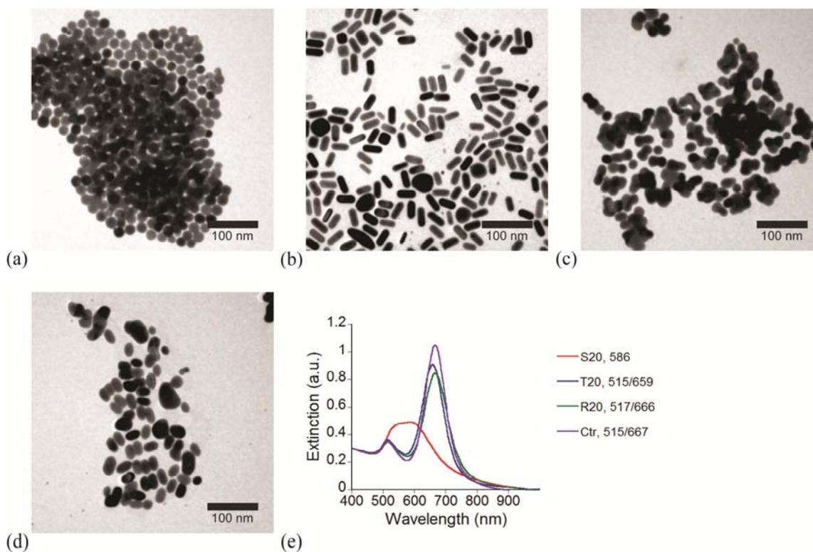
**FIG. S8.** TEM micrographs of 2  $\mu$ M incubation samples after 3 days (a) **S20** (b) **T20** (c) **R20** (d) Control= 2  $\mu$ L Tris HCl and (e) accompanying UV-Vis spectra of all incubation samples. The resulting peak wavelength values are included in the legend.
