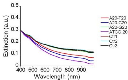
**FIG. S5.** UV-Vis spectra of gold seeds after a 2 h incubation in the presence of various homopolymer mixtures of two or four sequences at 2  $\mu\text{M}$ . Controls involve the addition of Tris HCl (Ctr1= 4  $\mu\text{L}$  Tris HCl, Ctr2= 8  $\mu\text{L}$  Tris HCl) or water (Ctr3= 4  $\mu\text{L}$  18 M $\Omega$ -cm water) in the absence of DNA.
