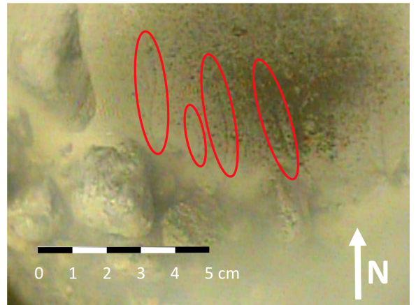
Fig. 11. Scratches in the hard granite bedrock in the borehole from 2017.
