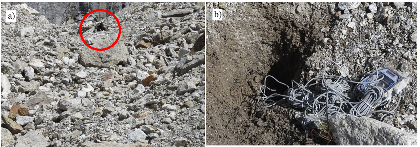
Fig. S2: a) Surrounding area of an example pit (SBP5). The red circle shows a person sitting near the pit. b) Pit SBP5 dug on Satopanth Glacier for temperature measurements. The temperature sensors are inserted on the pit wall and are connected to the data logger on the glacier surface.
