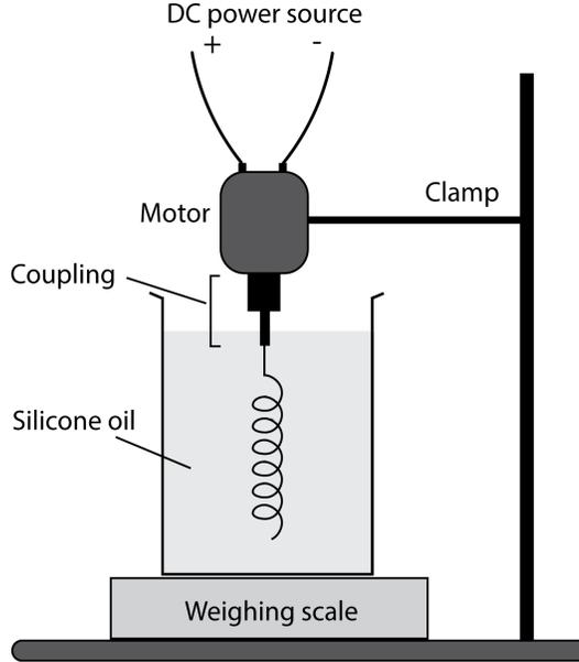
FIG. S1. Apparatus to study the propulsion by a rigid flagellum.
