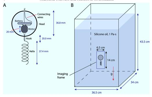
FIGURE 1. (A) A schematic of the model bacterium used in the experiments. (B) Dimensions of the tank and the approximate location of the bot during a run.
