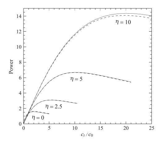
Comparison between analytical solutions (solid lines) and numerical model calculations (dashed lines) for the turbine dissipation, scaled with  $\rho h R^2 c_0 u_0^2$ , as a function of the non-dimensional turbine drag,  $c_t/c_0$ . The analytical curve for  $\eta = 0$  is from equation (3.3), while the curves for  $\eta > 0$  are from equation (4.1). Numerical results are from a linearized version of the model with vorticity advection omitted ( $\xi = 0$ ).
