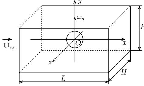
FIGURE SM 1. Sketch of the rectangular computational domain used in the DSMC simulations of transitional flow over a spinning sphere.
