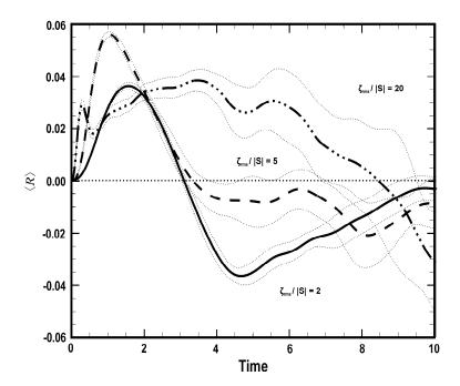
Time evolution of the ensemble mean Reynolds stress in decaying experiments with  $\zeta$  rms /| S|=(2,5,20) at t = 0 as discussed in §4.2. Thin lines represent the 95% confidence interval on the mean. This figure may be compared with results from the corresponding inviscid experiments presented in figure 8.
