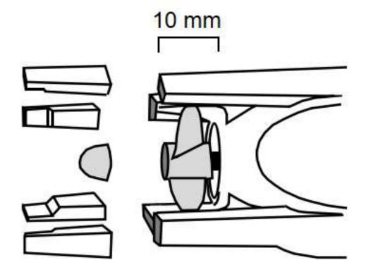
113 A pin of the propeller protection framework was removed.
