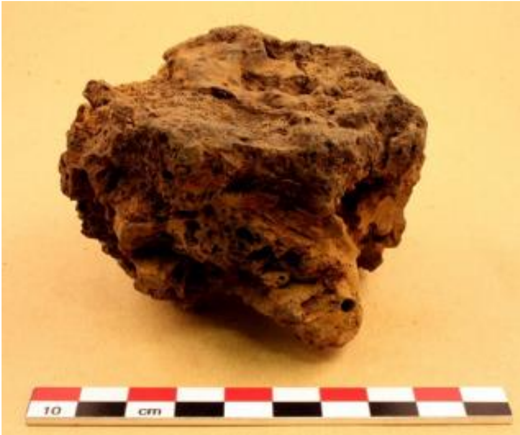
Figure S36. Bottom slag F83, seen from the side, with weakly bowl-shaped upper area (The Archaeologists, National Historical Museums, Uppsala, Sweden).
