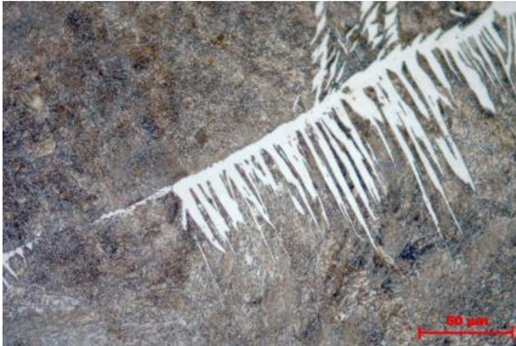
Figure S127. Id 2942. In very high magnification here the brown pearlite texture is seen with a grain boundary of carbon-free iron, ferrite, which shows feather texture (The Archaeologists, National Historical Museums, Uppsala, Sweden).
