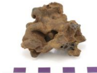
Figure S82. Slag id 2825 from slag heap in furnace area 2. Stearin slag, cemented sand below, moderately porous (The Archaeologists, National Historical Museums, Uppsala, Sweden).
