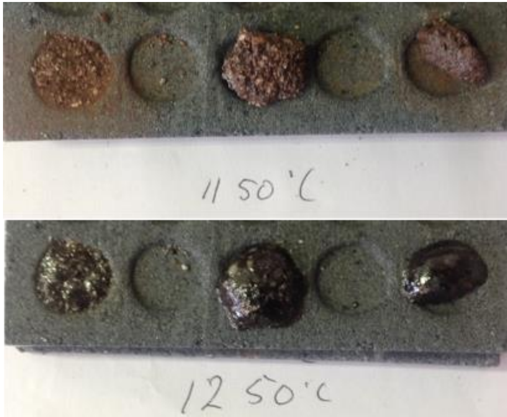
Figure S133. From left to right powder from clay samples I-III; Id 2854 and Id 1649 at 1150 and 1250°C respectively (A. Lindahl).
