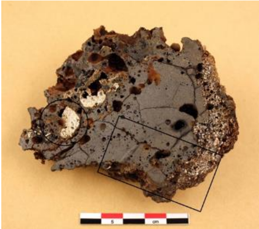
Figure S39. Slag F256 in cross section. The box shows the part of the slag that has been examined in the microscope. In the circle is the iron concentration that has also been analysed (The Archaeologists, National Historical Museums, Uppsala, Sweden).
