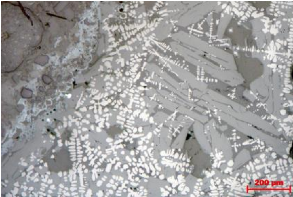
Figure S112. Id 2861. In higher magnification it is observed how the light wüstite grows dendritic over both grey olivine laminae and dark glass. Very small white iron drops can be perceived near the surface of the slag (left in the picture) (The Archaeologists, National Historical Museums, Uppsala, Sweden).
