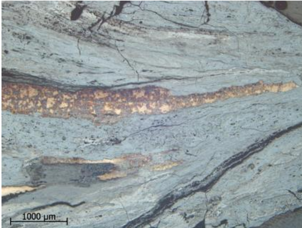
Figure S29. Find no. 2684. Micrograph of etched sample. Detail from the edge of the axe where it is mostly corroded (grey). A narrow band of metal is preserved. It consists of hardened steel (brown-blue shades) (The Archaeologists, National Historical Museums, Uppsala, Sweden).
