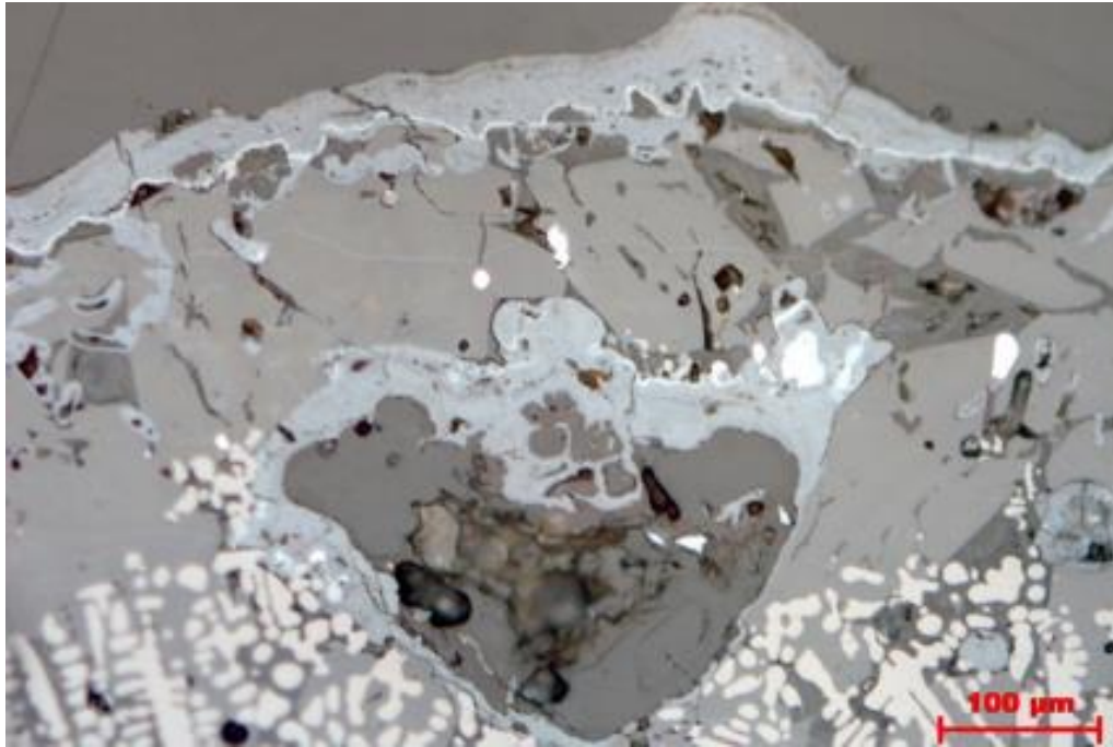
Figure S98. Outer edge of slag id 1809 in very high magnification where scattered white metallic iron drops can be observed. Note how the light wüstite is lacking in areas closest to the surface, which is ultimately covered by light grey rust/iron hydroxide. This may be due to high presence of oxygen at the formation of the slag (The Archaeologists, National Historical Museums, Uppsala, Sweden).
