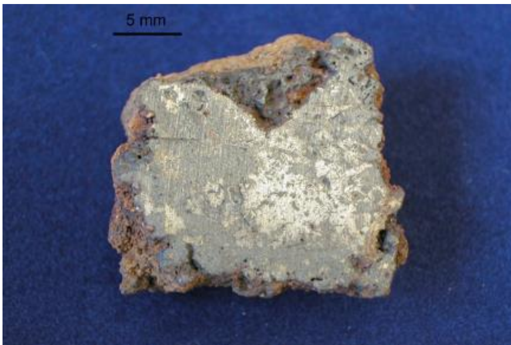
Figure S18. Find no. 922 from A4. Spongy iron (light) and slag (darker) (The Archaeologists, National Historical Museums, Uppsala, Sweden).
