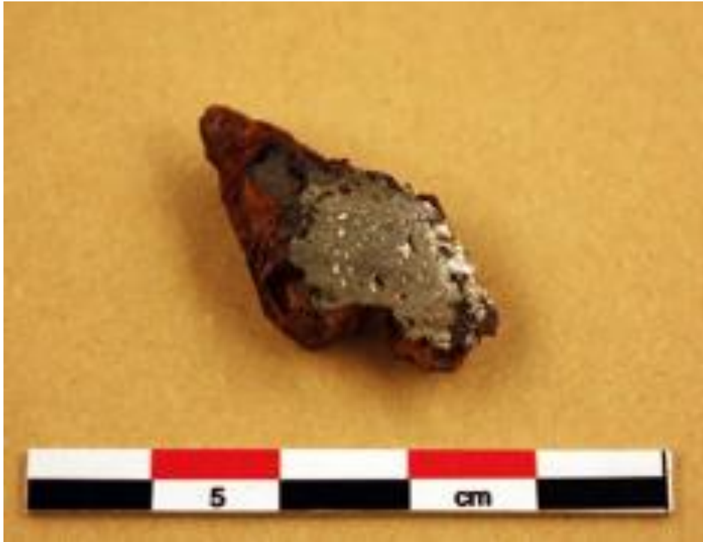
Figure S57. F759 in cross section. Concentration of metallic iron which is rather dense (The Archaeologists, National Historical Museums, Uppsala, Sweden).
