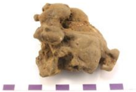
Figure S89. Slag id 2861 from the furnace chamber in furnace area 3. Scattered charcoal imprint, porous, has flowed (The Archaeologists, National Historical Museums, Uppsala, Sweden).
