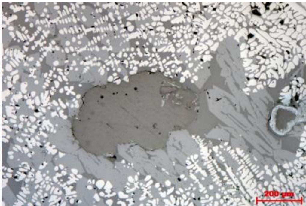
Figure S106. Slag id 1973 in high magnification. It shows how the light wüstite grows dendritic over both the grey olivine laminae and the dark intermediate matrix, which probably consists of glass (The Archaeologists, National Historical Museums, Uppsala, Sweden).
