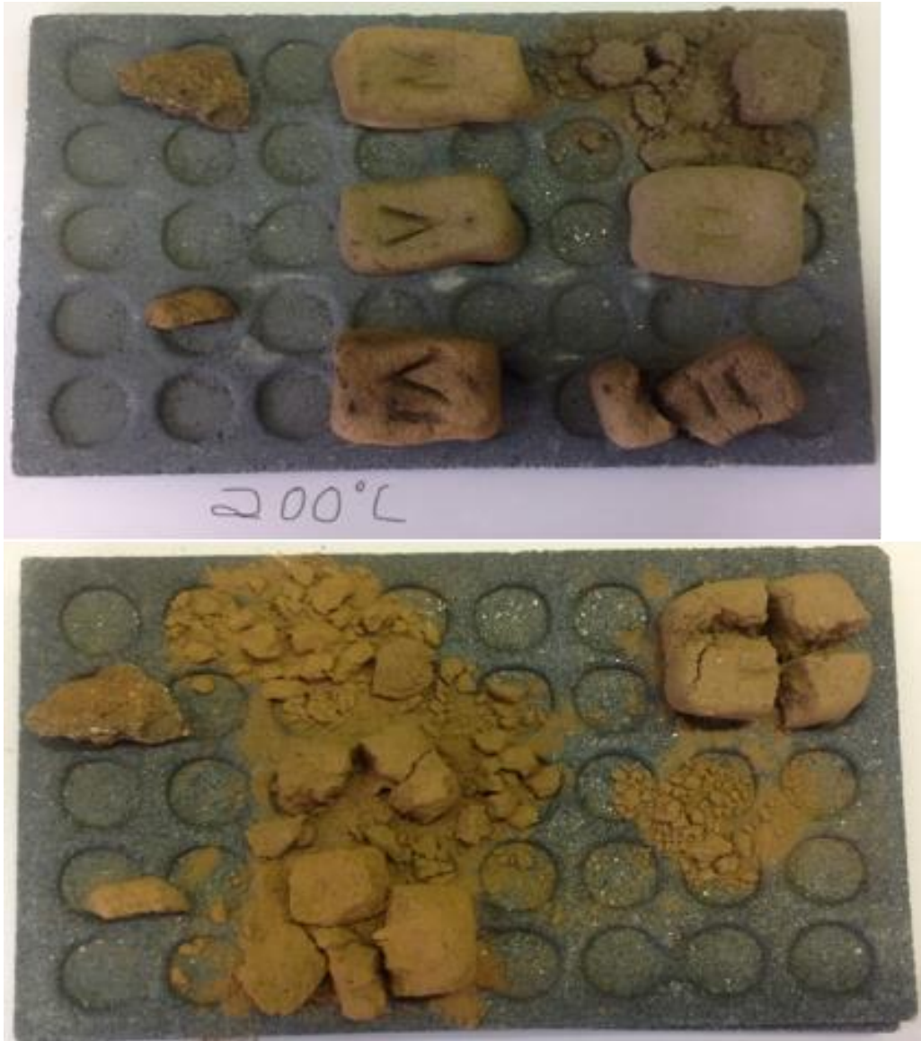
Figure S132. Photos of the clay samples' condition after 200 and 500°C (below) compared with the two furnace wall fragments to the left (A. Lindahl).
