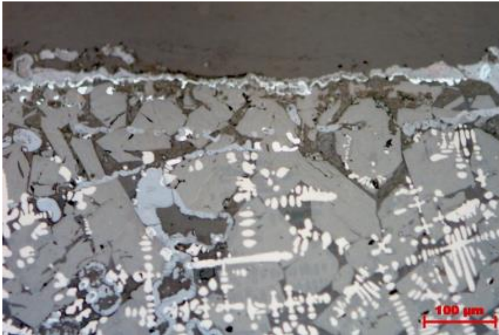
Figure S104. Slag id 2825 in high magnification. Sparse metallic iron is perceived as very small white drops, mainly close to the surface of the slag. The presence of light wüstite decreases next to the surface of the slag, where instead grey olivine crystals and dark glass dominate (The Archaeologists, National Historical Museums, Uppsala, Sweden).
