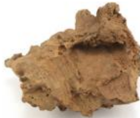
Figure S86. Slag id 1973 from slag heap in furnace area 3. Low viscosity, charcoal imprint, relatively dense (The Archaeologists, National Historical Museums, Uppsala, Sweden).
