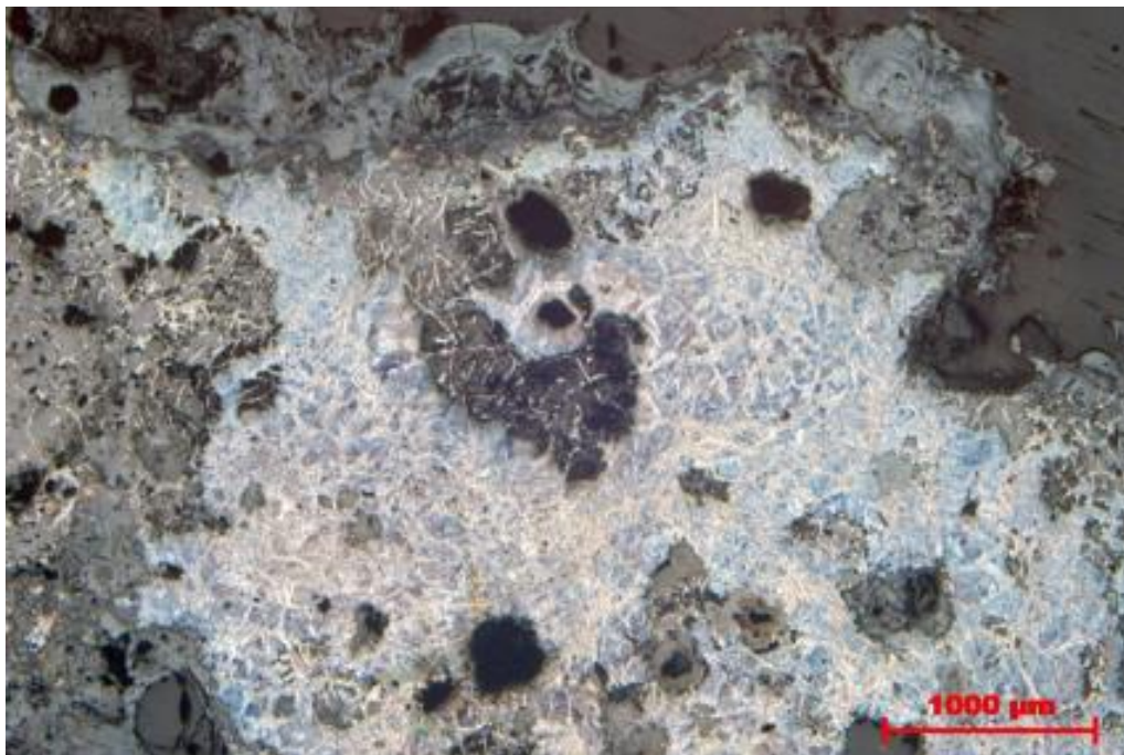
Figure S118. After etching of iron sample id 392 it appears that the carbon content is high. The sample consists of pearlite and cementite (The Archaeologists, National Historical Museums, Uppsala, Sweden).
