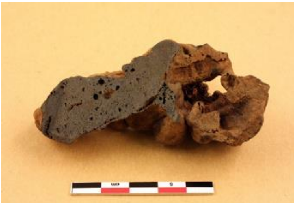
Figure S33. F930, stearin slag in cross section with a few small pores (i.e. a dense slag) (The Archaeologists, National Historical Museums, Uppsala, Sweden).
