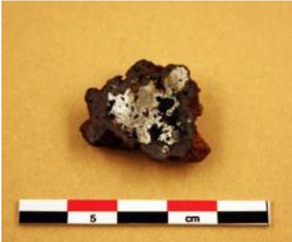
Figure S63. Id 243. Concentration of metallic iron with slag inclusions as well as cavities and corroded areas (The Archaeologists, National Historical Museums, Uppsala, Sweden).
