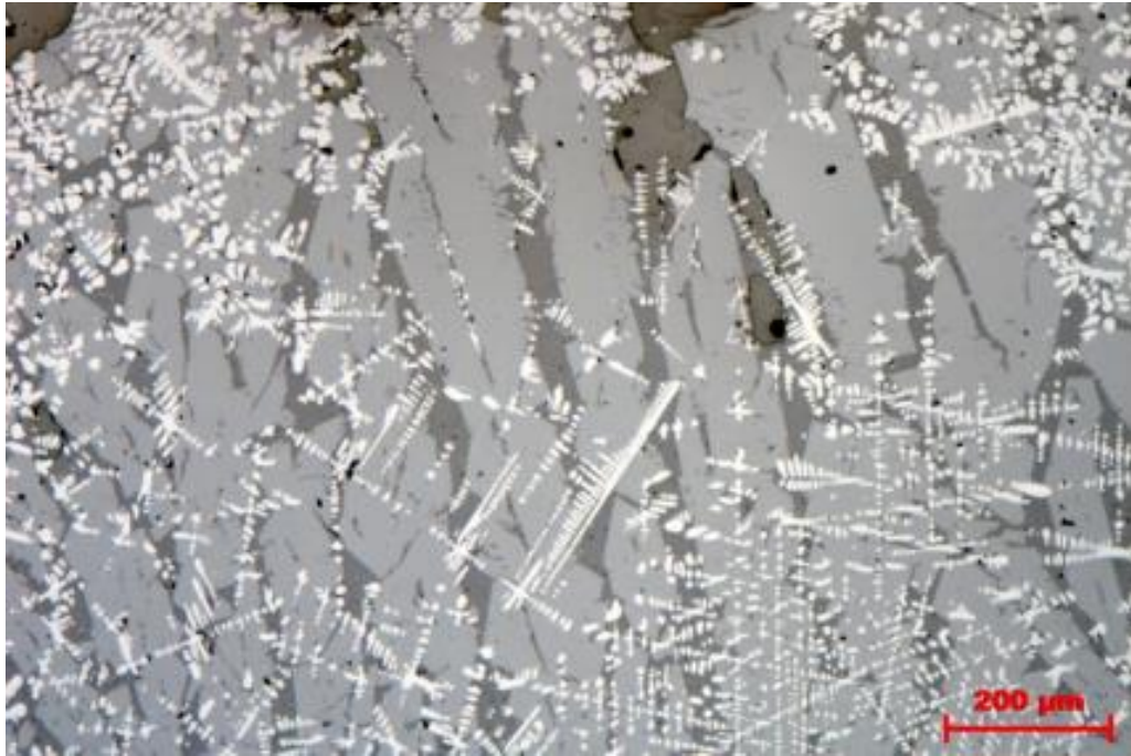
Figure S110. Id 2854. In higher magnification the dendritic light wüstite is seen to grow over both grey olivine and dark glass (The Archaeologists, National Historical Museums, Uppsala, Sweden).
