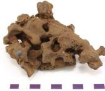
Figure S80. Slag 1809 from slag heap in furnace area 2. Stearin slag, cemented sand below, relatively dense (The Archaeologists, National Historical Museums, Uppsala, Sweden).
