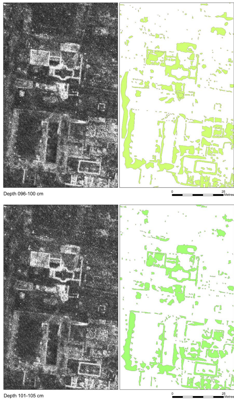
Figure S8. GPR time-slices from the sample area at Falerii Novi (for location see Figure 4) at depths 096–100cm and 101–105cm: left) GPR image; right) manually mapped anomalies (illustration: A. Launaro; GPR data: L. Verdonck).
