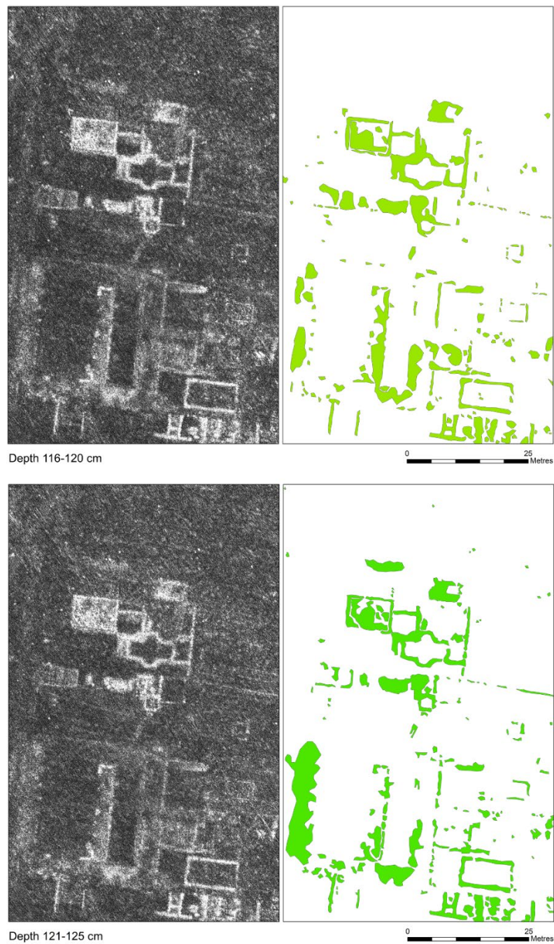
Figure S10. GPR time-slices from the sample area at Falerii Novi (for location see Figure 4) at depths 116–120cm and 121–125cm: left) GPR image; right) manually mapped anomalies (illustration: A. Launaro; GPR data: L. Verdonck).
