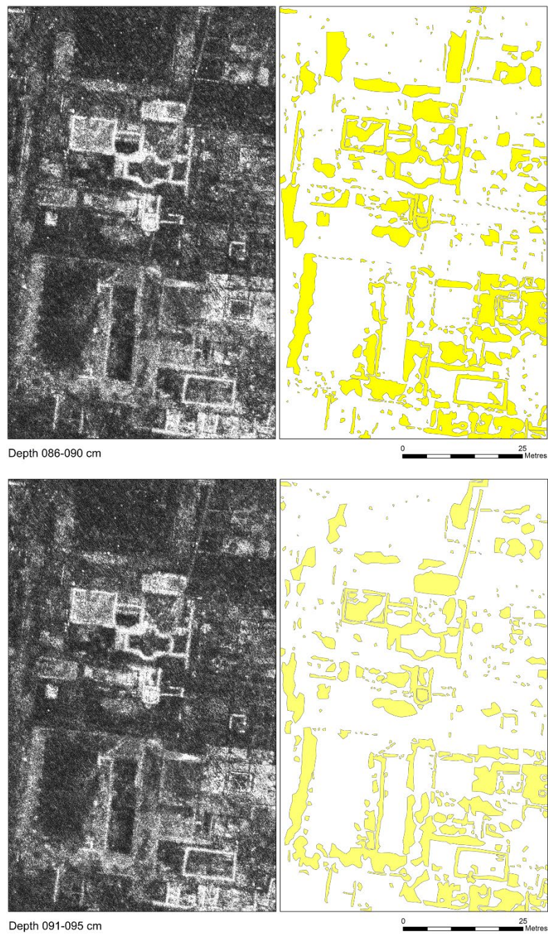
Figure S7. GPR time-slices from the sample area at Falerii Novi (for location see Figure 4) at depths 086–090cm and 091–095cm: left) GPR image; right) manually mapped anomalies (illustration: A. Launaro; GPR data: L. Verdonck).
