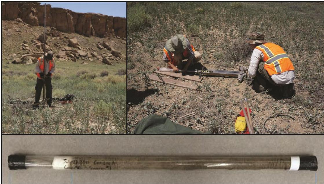
Figure S2.1. In field extraction of a polyethylene terephthalate plastic lined soil cores. Top left: Hammering the core into the sediment; top right: removing core sections from the coring machine; bottom: labelled core section following extraction. Figure created by the authors.
