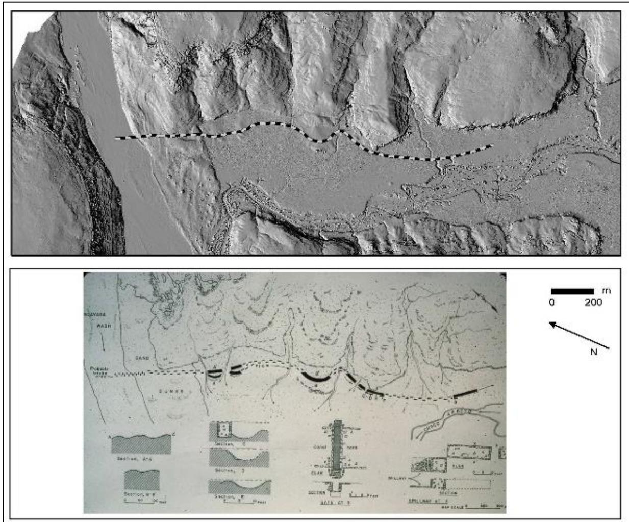
Figure S7.1: The Gordon Vivian hypothesized canal (c.1964) feeding from Escavada Wash, thru the dune and up Chaco Canyon. The Vivian map (CHCU-55430 1971; *pers. comm.* Gwinn Vivian 2015), bottom image, is aligned with the lidar-derived hillshade image above. The Vivian canal line is transposed to the lidar map. Our excavations were in the “A” section of the postulated canal. Figure created by the authors.
