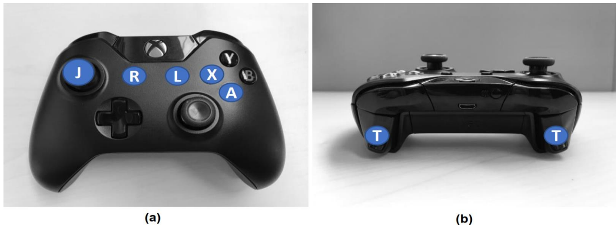
Figure 7: The Xbox controller: (a) shows the top view with the left-hand joystick [ J ] used to control the 2D movement on the X-Z plane whereas (b) shows the front view with the two triggers [ T ] responsible for vertical movement along the Y axis. The other action buttons indicated in (a) have the following meanings: [ R ] for reload of the visualization; [ L ] for loading next dataset; [ A ] for selection of an interactive item; and [ X ] for moving or rotating
