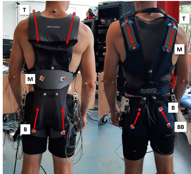
Fig. A.1. Soft exosuits apply forces parallel to the trunk. The direction and point of application of forces generated by the exosuit (red arrows). The stretch of the exos were measured using markers placed (red dots) for the Darwing (left) and Auxivo (right). In case of the Darwing, the elastic bands were 65% the distance between T and M markers.
