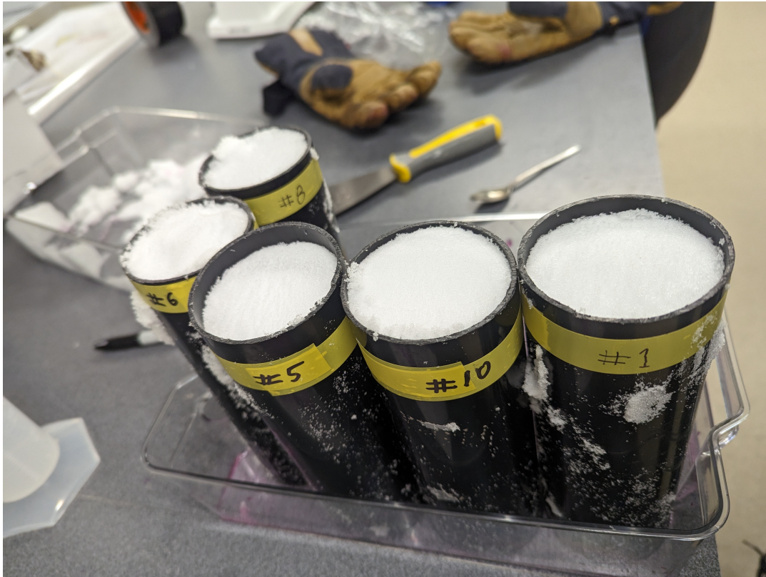
Fig. S3. Photograph showing the previous setup of the experiment, where snow samples and their tubes ‘shared’ a brine supply. This led to preferential uptake from some samples and led to unreliable results.
