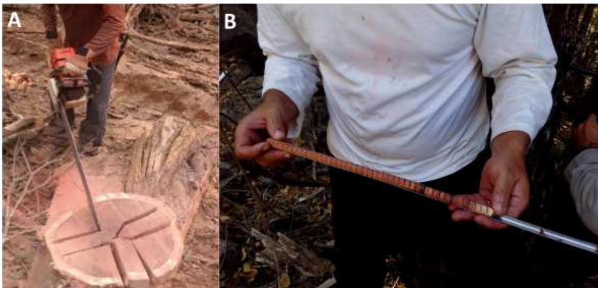
Figure S2. Images of basic tree-ring sampling methods, such as (A) cross-section, and (B) increment core.
