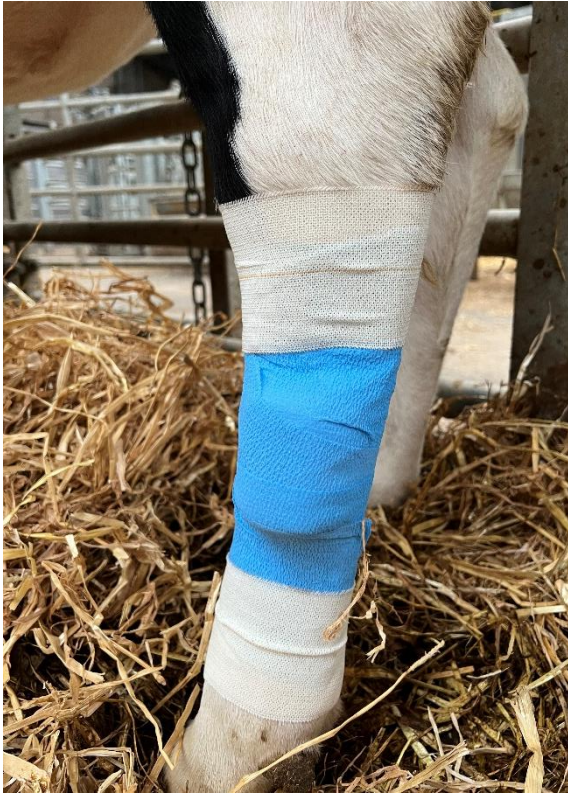
Supplementary Figure S1: Demonstration of IceTag application to the lateral aspect of the hindlimb of one calf using cohesive bandage (Wrapz®, Millpledge Veterinary, UK) and elastic bandage (Tensoplast®, BSN Medical, UK).
