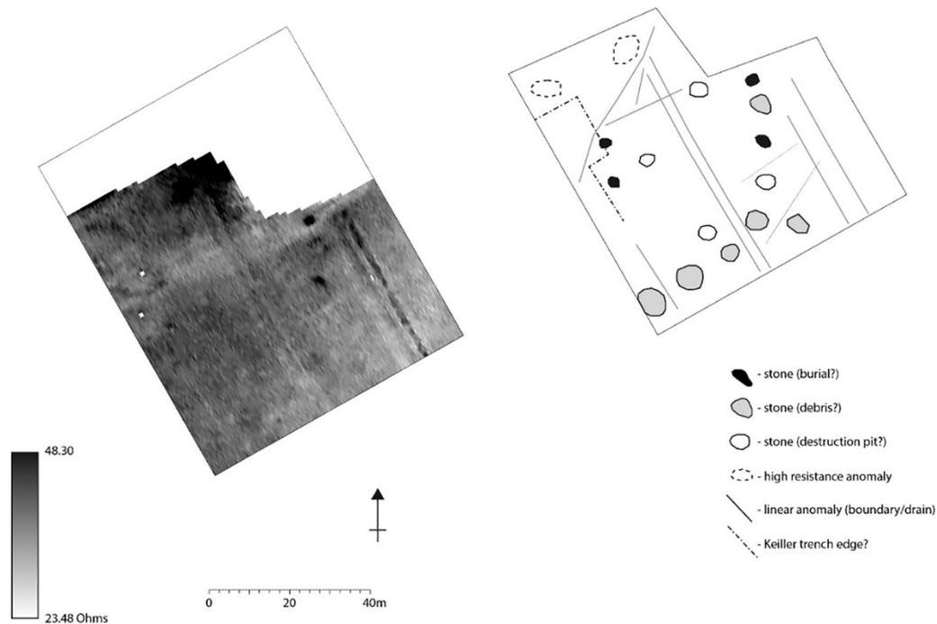
Figure S3. The twin-probe resistivity results (displaying +/- 3 standard deviations).
