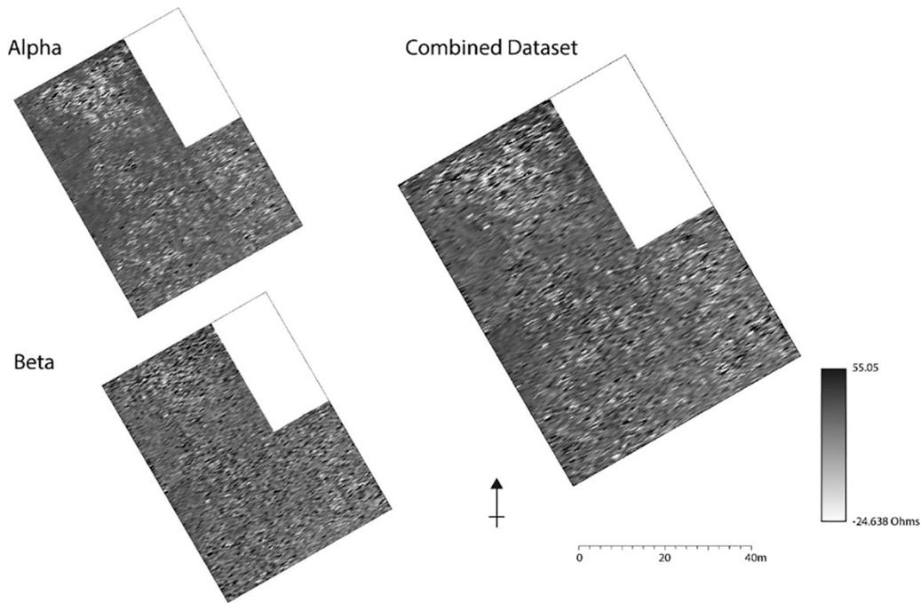
Figure S5. Square array resistivity data—Alpha, Beta and combined datasets.
